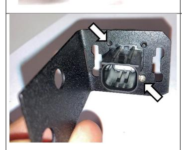
3. Reinstall the camera into the included bracket (3753977) and fasten with the two original phillips head screws.
